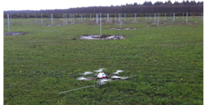
Fig. 1. Partial view of the LBA array. The UAV equipped with a 2-m long dipole is taking off
