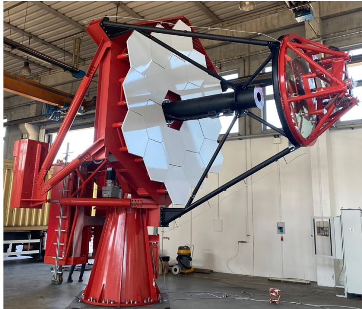
Figure 2 left: a 3-D model of the SST telescope structure; right: the first ASTRI Mini-ray telescope fully assembled in a warehouse in Italy before being shipped to the Tenerife Canary Island. This is also the baseline of the SST telescopes, currently under study for further possible improvements.
