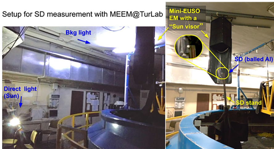
Fig. 26 TurLab setup for SD detection by the Mini-EUSO EM. The FS of Mini-EUSO EM apparatus is protected by a “Sun visor” to avoid the direct light from the white LED which is fixed outside of the tank, mimicking the Sun light. An Aluminum-ball under the apparatus of Mini-EUSO EM is attached to a solid stand which is fixed to the bottom of the tank. As the tank rotates, the Aluminum-ball moves within the EUSO@TurLab apparatus FoV being illuminated by the LED. Image adapted from [36]
