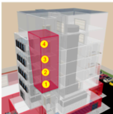
Figure 1-39. Building volume dedicated to the technical rooms.
