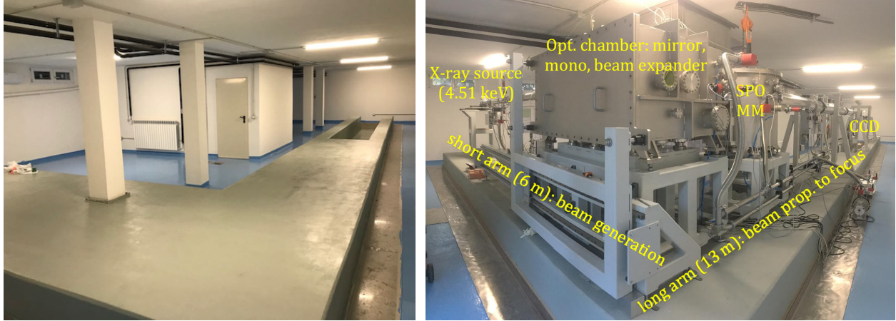
Figure 3: the status of the BEaTriX lab in May 2020 (left) and in July 2021 (right). All the vacuum system was realized and installed by Kenosistec (Binasco, Italy) in a building basement and mounted on an anti-vibration platform. The chambers enclose the optical components that will expand and parallelize the X-ray beam. All the system fits within 17\text{ m} \times 8\text{ m} .
