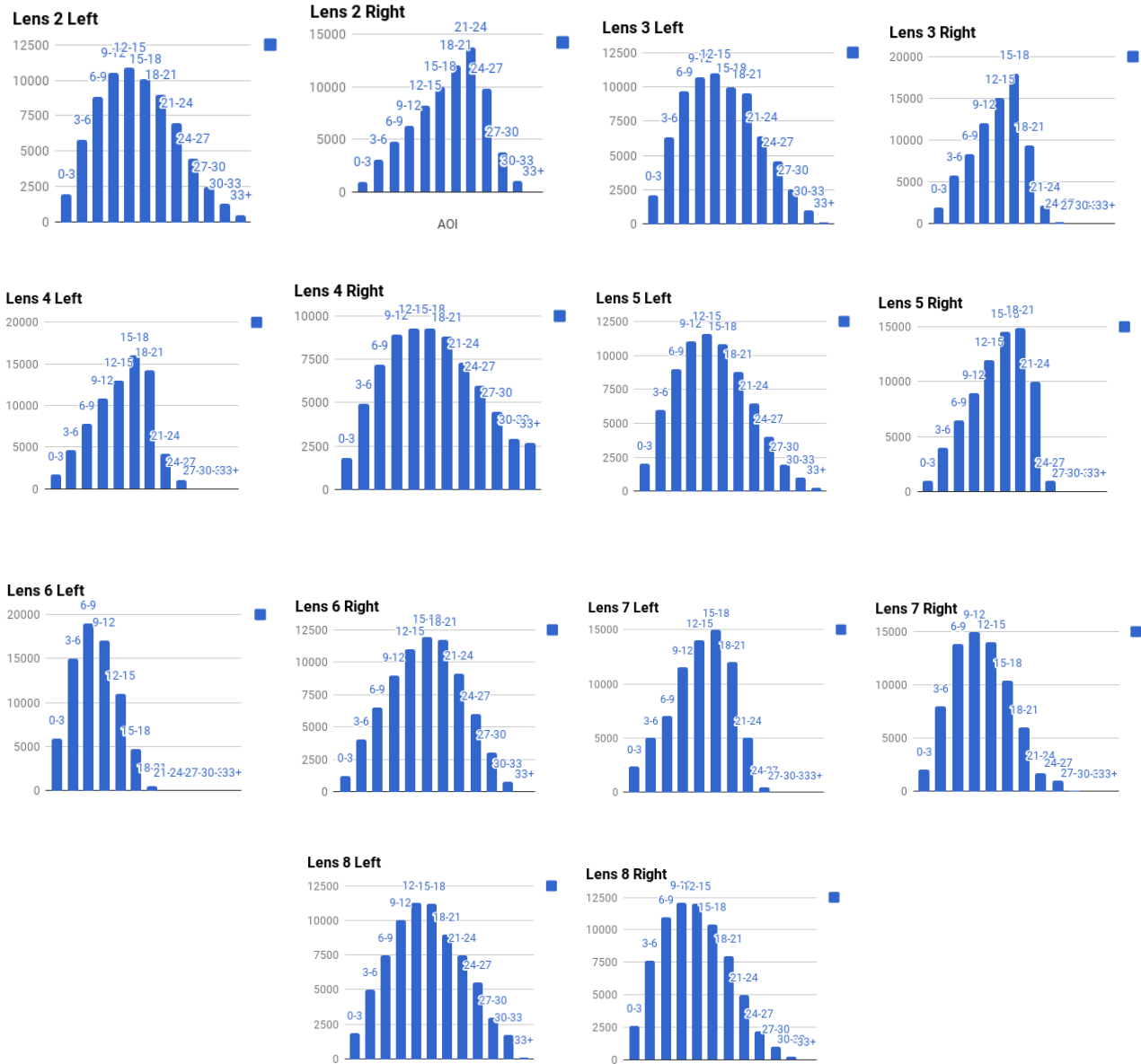
Figure 1. Histograms of number of rays hitting the indicated lens surface at different AOI bins.
