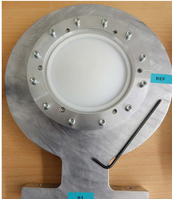
Figure 9. Lens mounted on S1. See the reference sign on the right of the support as seen from the front.
