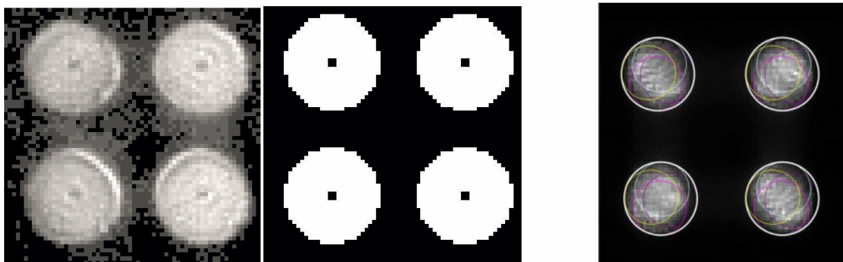
Figure 5. On the left, a frame from the the CCD50 on the GWS WFS looking on a single fiber with AdSec applying the flat shape. On the central panel: the pupil mask as encoded in the Real Time Computer (RTC) software. Here the system used a 2 \times 2 binning on chip, the same used for on sky operations in the case of bright reference stars. On the right the CCD39 is focused in order to make the super imposition of the pupil covering the metapupil (or the Xinetics DM).
