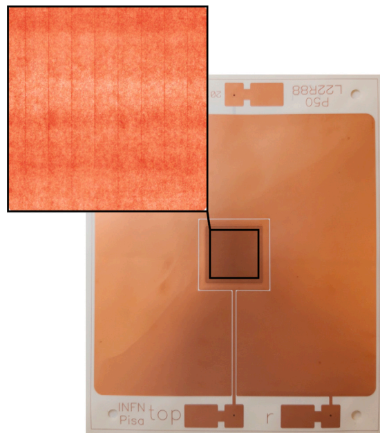
Fig. 5. Photograph of a flight model GEM. The active area is the darker region in the center, while the rest of the copper is the guard ring on the top surface. The soldering pads for the high-voltage cables are visible on the very top and the very bottom of the image. The micro-photograph of the GEM active region shows the (vertical) features in correspondence to the sweep overlaps at the laser drilling stage, as explained in the main text. We emphasize that the second pass of the laser etching, in the orthogonal direction, is performed from the opposite side of the GEM, and therefore the horizontal features are not visible on the top surface pictured in the inset.
