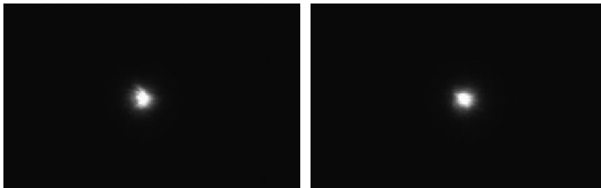
Figure 12: First two images (from a 60 s sequence) taken with the Aqueye+ field camera on Nov 19, 2014 (start time 05:48:50.6). The exposure time is 10 ms and the capture time interval 0.1 s.
