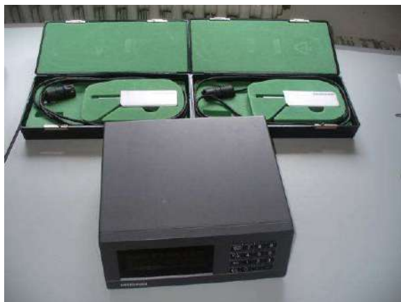
Figure 6-17: Heidenhain sensor for the rotation calibration
