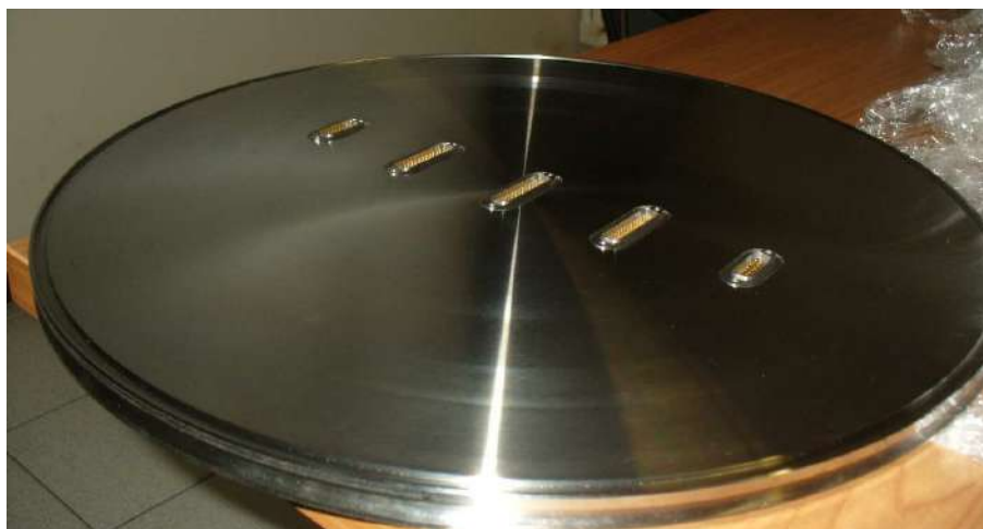
Figure 6-18: PANTER flange with dedicated connectors
