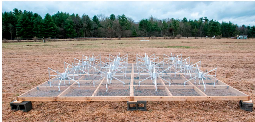
Figure 2. (a) Reference antenna on 2\text{ m} \times 2\text{ m} ground screen (see section 2.3) and (b) MWA antenna tile on 5\text{ m} \times 5\text{ m} ground screen (see section 4) deployed at the National Radio Astronomy Observatory–Green Bank.
