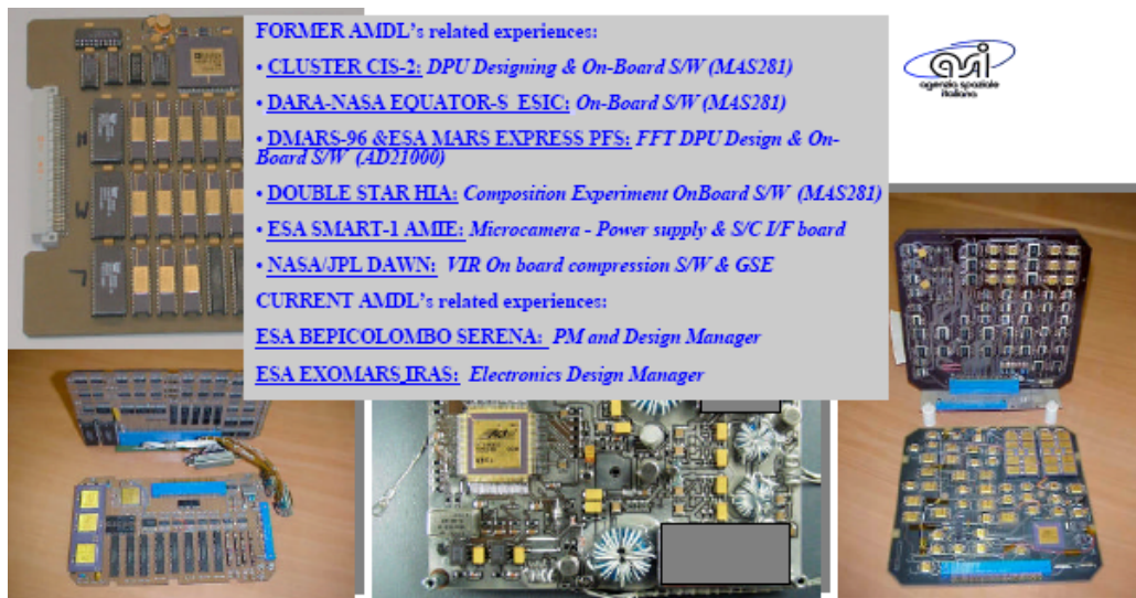
Figure 1.3. Flight DPU inheritance for SCU development. Collection of boards snapshots developed in the frame of space mission supported by AMDL Srl in cooperation with INAF/CNR Upper Left Panel: Engineering model of MARS96 and MEX Planetary Fourier Spectrometer FFT DSP board for which AMDL Srl supported H/W and S/W; Bottom Left Panel: Engineering model of CLUSTER Cis-2 Spectrometer CPU and I/F boards for which AMDL Srl supported H/W and S/W; Bottom Center Panel: SMART-1 AMIE Camera, Power Supply and S/C I/F board for which AMDL Srl supported H/W; Bottom Right Panel: Equator-S ESIC S/W development DPU boards (for which AMDL Srl supported software).
