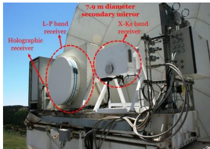
Figure 3. Photo of the Front-Ends at the SRT primary focus. The L-P band receiver is located between the X-Ka band and the holographic receivers. All Front-Ends are mounted on the primary focus positioner (PFP), a robotic arm that brings the Front-Ends at its focal position during primary focus observation. The 7.9-m diameter quasi-ellipsoidal secondary mirror is visible in the back.
