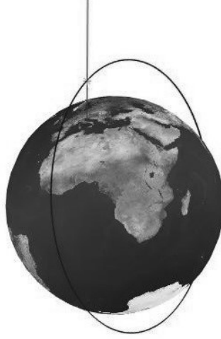
Figure 14: Intersection between the line connecting the ground station to the observed object position and the orbital plane
