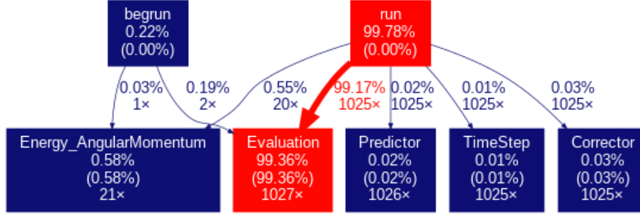
Fig. 1: Call graph of HY-NBODY profiled using gprof tool. The figure shows nodes and edges above the threshold 0.01.
