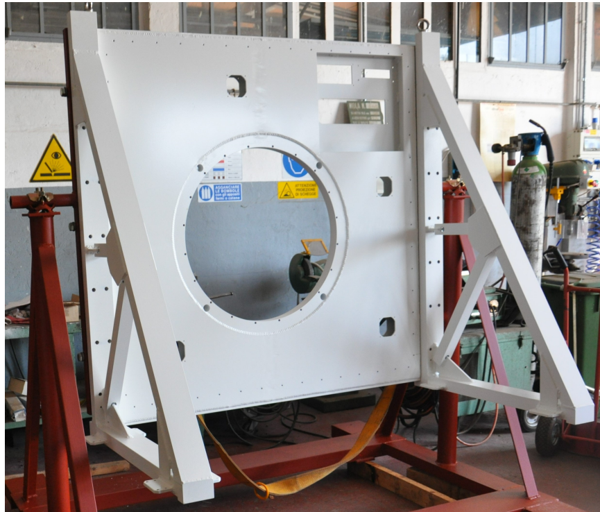
Figure 4. Current frame structure for the L-P band receiver
