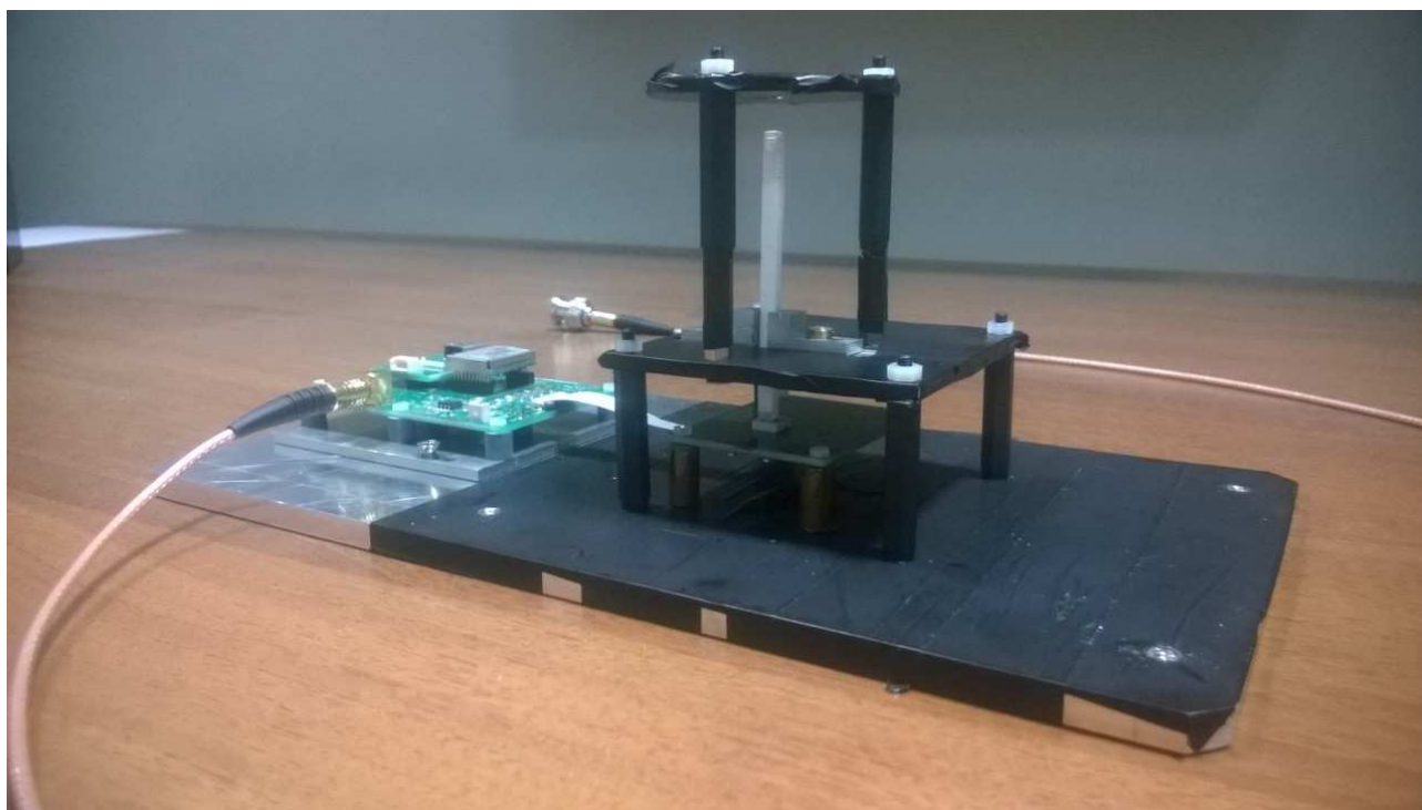
Figure 6: Picture of the experimental set-up. The power supply board is on the left, connected with the flat cable to the sensor board (center). The SiPM is placed on the sensor board. In the picture, the detector on top of the SiPM is a plastic scintillator rod. The light tight box to cover the sensor board and the mechanical structure is fixed to the four threaded holes. The black tape is used to reduce the reflection of stray light from the environment.
