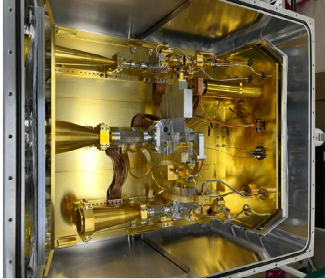
Figure 2. Picture of the passive components inside the cryogenic chamber. The three feedhorns are visible in the left side of the photo.
