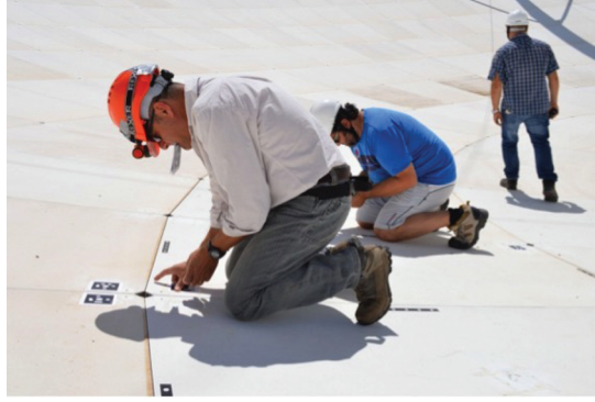
Figure 2. Setting up photogrammetric measurements at the SRT.
