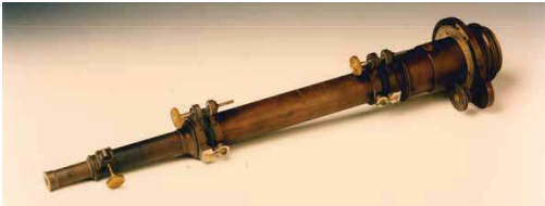
PA.03. ZÖLLNER-TYPE DIRECT-VISION SPECTROSCOPE M. Tauber, Leipzig (Germany), ca. 1870 brass, steel, glass; total length 550 mm INAF-Palermo Astronomical Observatory*
