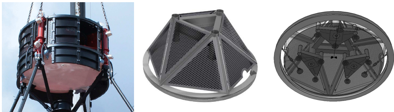
Fig 7. M2 BUS for prototype (left) and for array telescope (centre and right)
