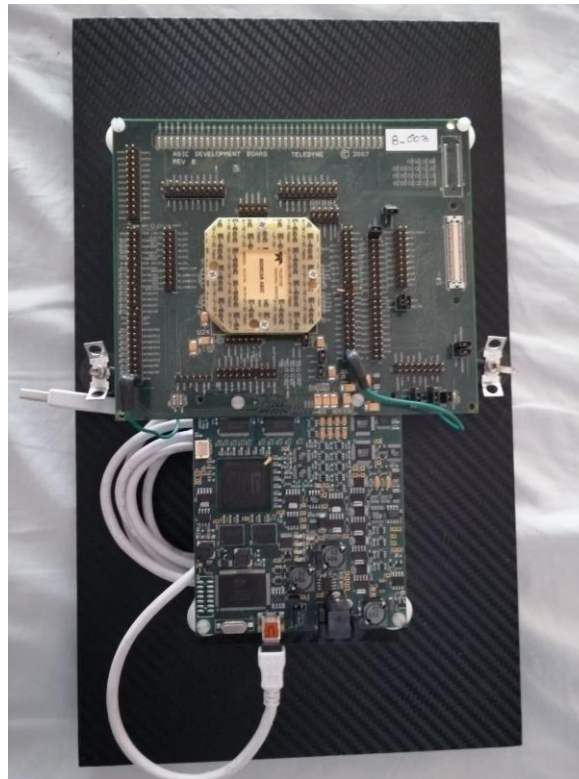
Figure 9, JADE stand-alone SCE readout system.
