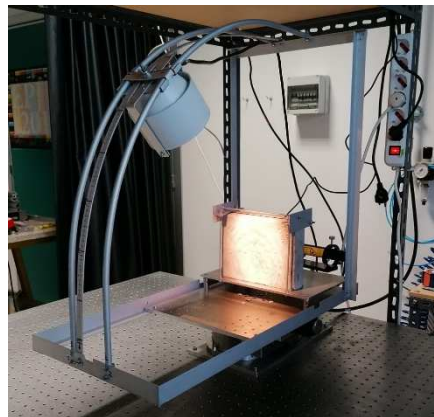
Figure 8. The stone illuminated by a halogen lamp used as HYPSSOS source.
