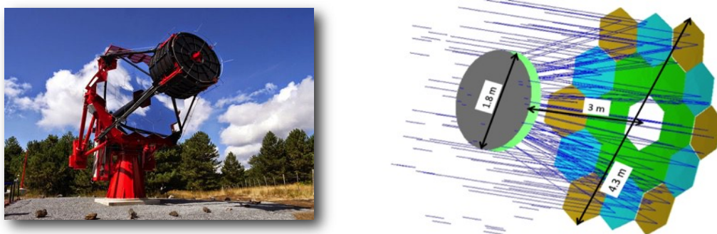
Figure 1 – Left: picture of the ASTRI SST-2M telescope installed at Serra la Nave (Catania, Italy), Right: sketch of the ASTRI Schwarzschild-Couder dual mirror optical design
