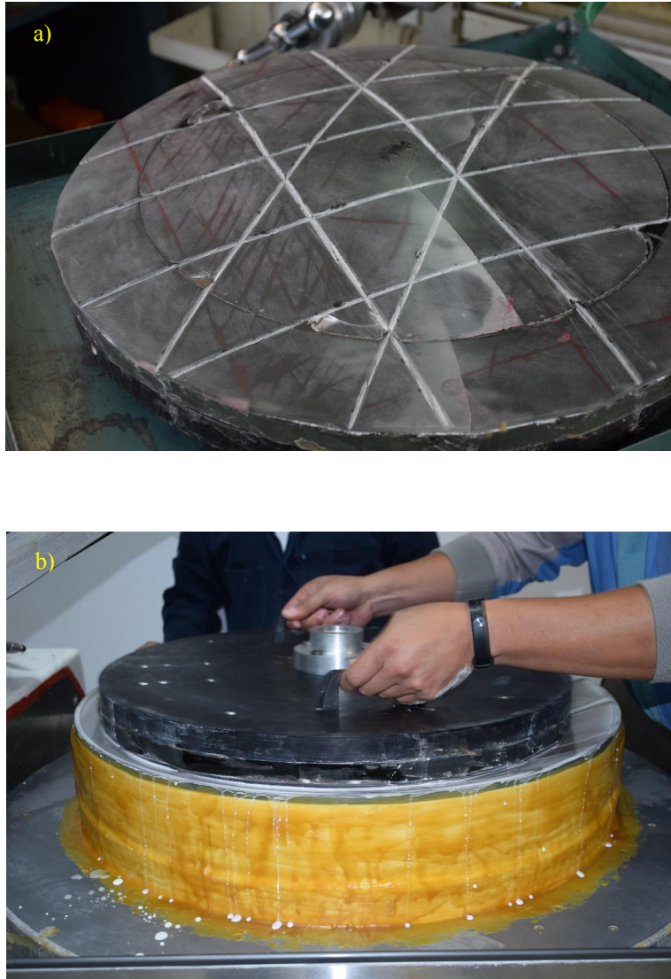
Figure 7. (a) Detail of the grinding glass tool of 560 mm diameter. (b) Grinding process.
