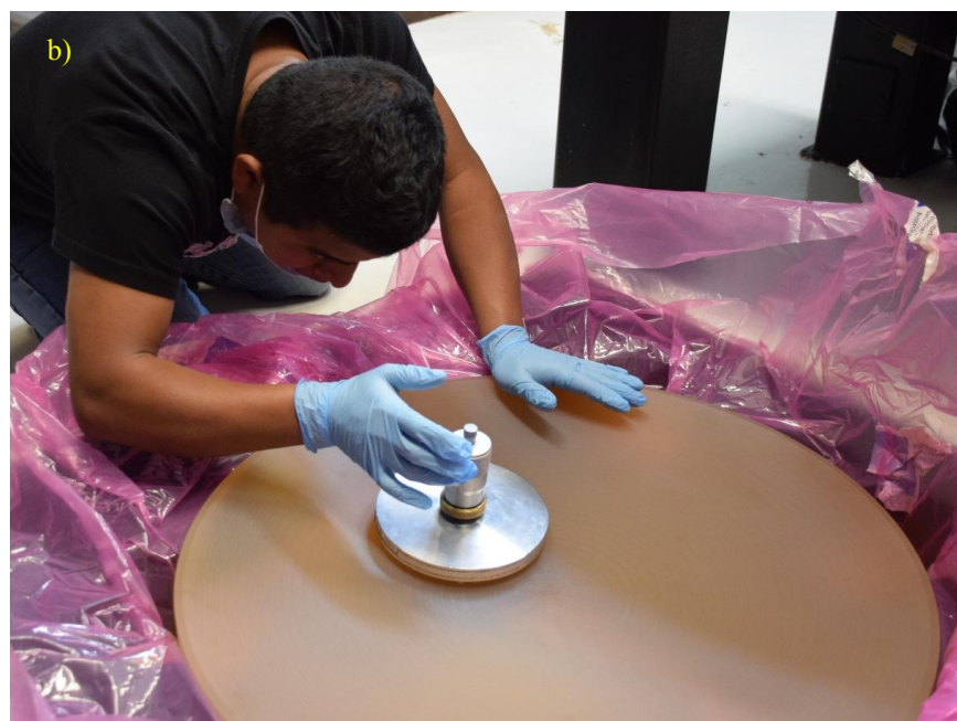
Figure 3. (a) Collimator blank verification. (b) RoC initial measurements.
