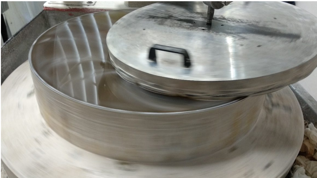
Figure 8. (a) Detail of the polishing pitch tool, 600 mm diameter. (b) Polishing process.
