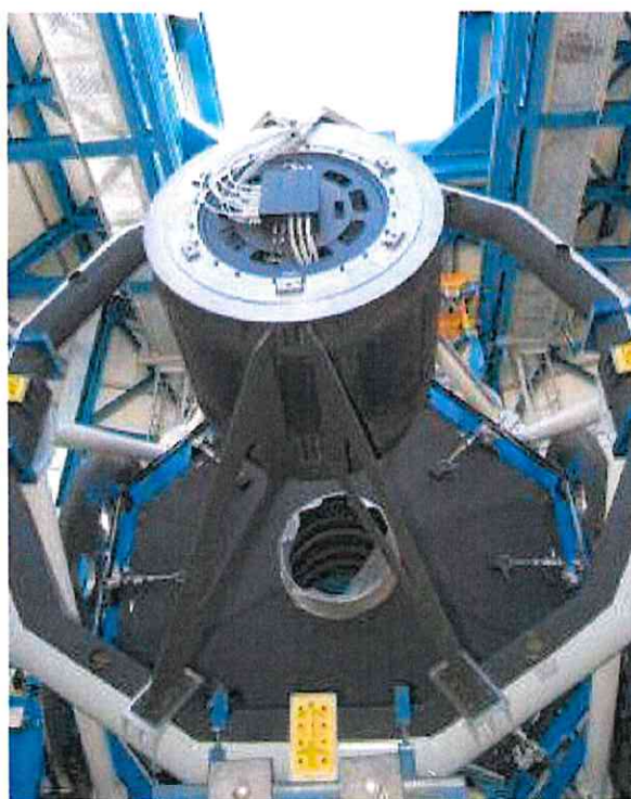
Fig. 7 – The secondary mirror support system integrated in the telescope in Chile.
