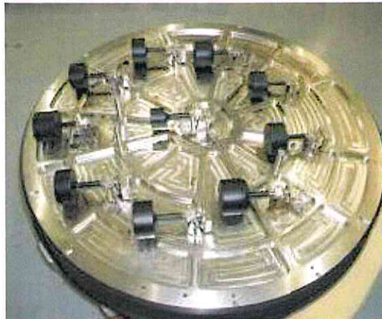
Fig. 4 – The astatic lever support system during the integration
