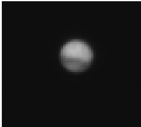
Figure 15 First Image of Mars acquired during the Mid cruise check in 13 June 2016 (41 Millions kilometers from Mars). The image confirms in base of the pixel scale that from this distance Mars appears around 15 pixels (11.36 arcsec/pixel)
