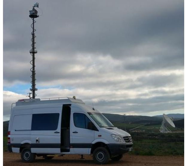
Figure 2. RFI mobile laboratory during an RFI monitoring at a measuring station close to SRT (in background).
