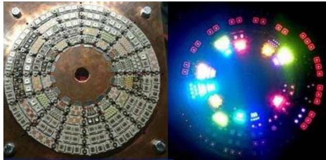
Figure 2: LEDs as mounted on the board (left) and illuminated (right).
