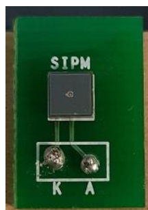
Figura 3. SiPM LVR3 S14160-3050TSV 3 \times 3 \text{ mm}^2 con microcella da 50 \mu\text{m}
