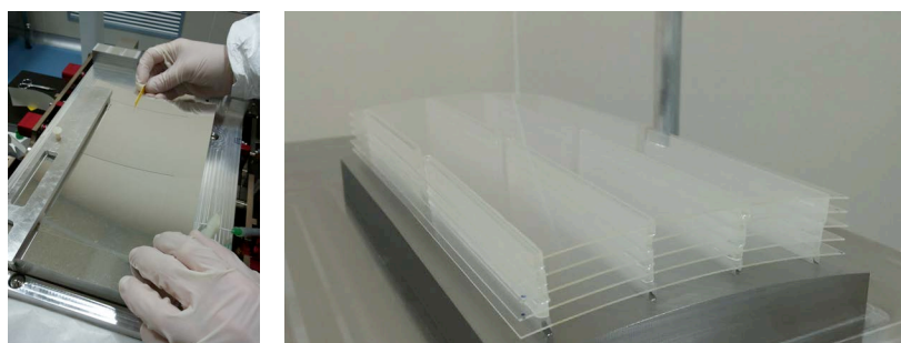
Figure 2: (A) Monolithic concave mold dedicated to the integration of indirect slumped glass provided by MPE. (B) JIM prototype made in 2015 with 5 glass layers.
