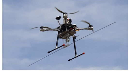
Fig. 3. UAV-mounted dipole hovering during the measurement.
