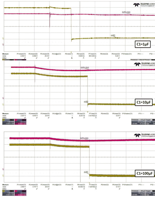
Figure 14: Variation in OC detection time when varying load capacity
