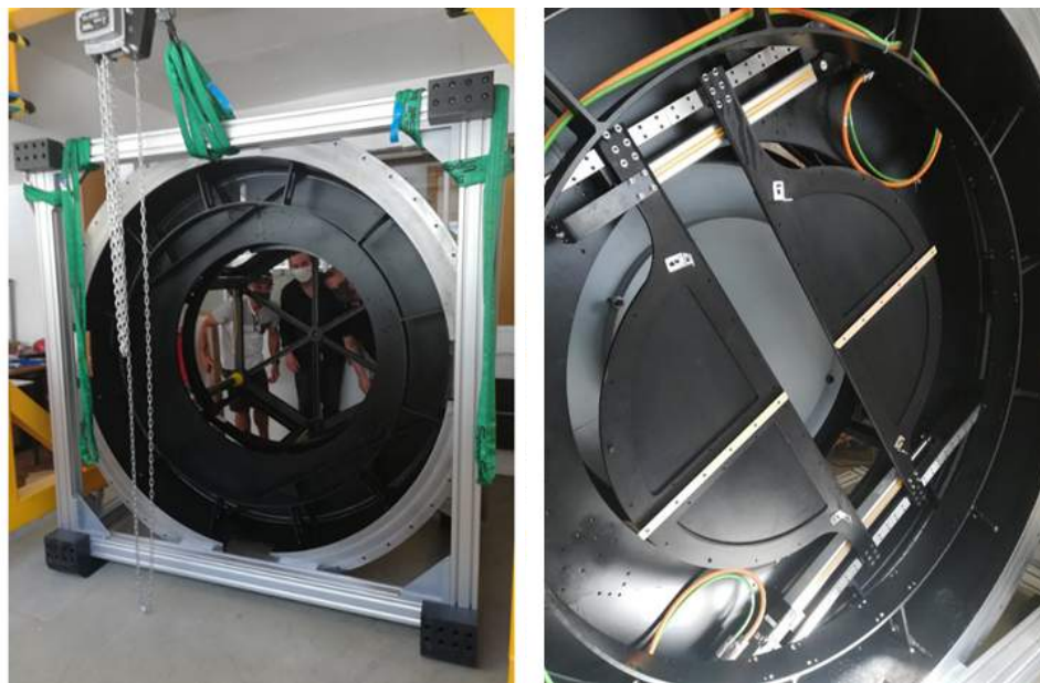
Figure 3. Rotating front end structure during integration and tests of the retraction and screen mechanisms
