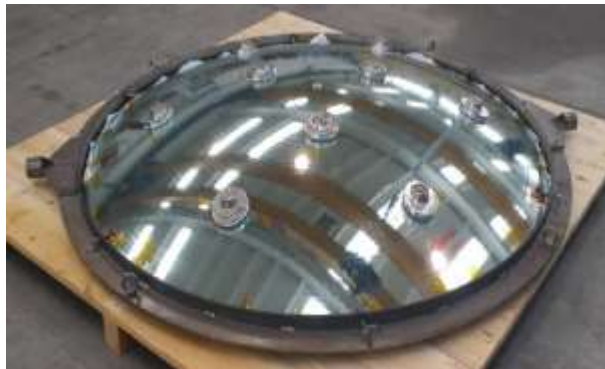
c) ASTRI M2 with I/Fs to the telescope
