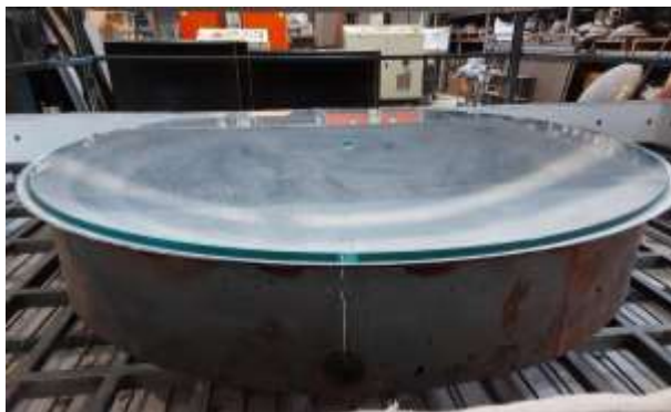
a) ASTRI M2 metallic mould + flat glass sheet
