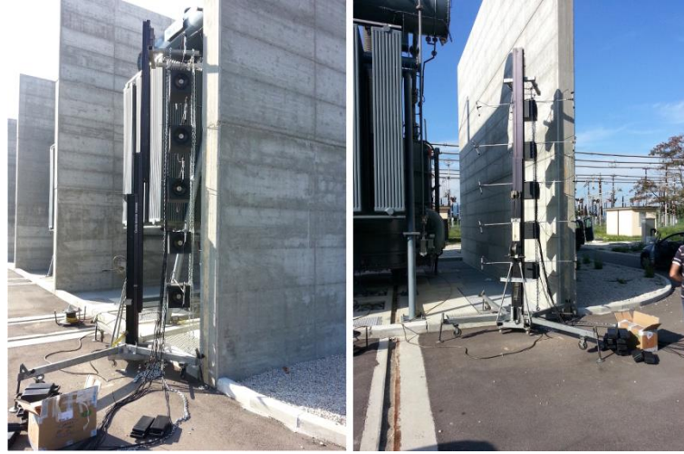
Figure 12 - Deployment of the ANC system at an electricity generation station in Tuscany (Italy).
