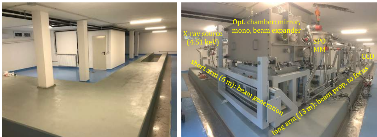
Figure 3: the status of the BEaTriX lab in May 2020 (left) and in July 2021 (right). All the vacuum system was realized and installed by Kenosistec (Binasco, Italy) in a building basement and mounted on an anti-vibration platform. The chambers enclose the optical components that will expand and parallelize the X-ray beam. All the system fits within 17\text{ m} \times 8\text{ m} .
