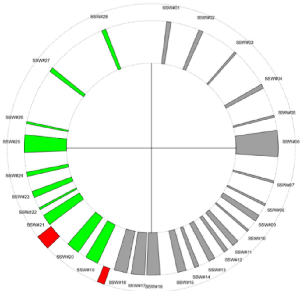
Fig. 7. DREAMS mission timeline for operation in day 1 showing sensor activation windows (in green) after expected landing and orbiter passage timelines (in red) in Mars local Time. (For interpretation of the references to colour in this figure legend, the reader is referred to the web version of this article.)
