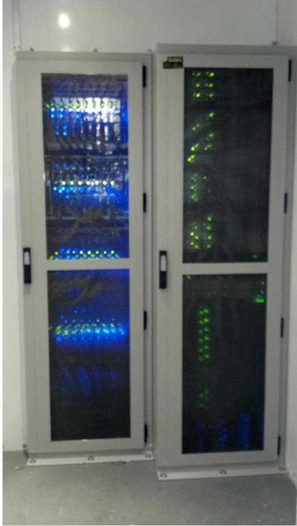
FIG. 5.— Front view of LEDA correlator racking (right). Large-format EMI air filters adopted to enable most readily the front-back airflow required by the digital hardware comprise the door. Screening at 40 MHz is \sim 50 dB. The lefthand rack contains high-gain analog electronics and is independently shielded against RF interference. RF-tight pass throughs in the common wall convey signals from the analog electronics to the correlator digital samplers. The setup is conceptually similar to that adopted for LWA1 (Taylor et al. 2012; Ellingson et al. 2013) though more compact and capable of supporting greater power and computational density.
