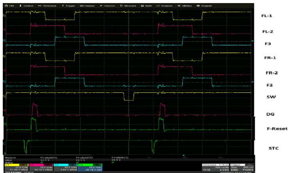
Figure 6. CCD horizontal phases and control timing.
