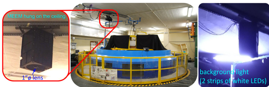
Fig. 3 The TurLab tank setup with the Mini-EUSO EM installed on the ceiling and enlarged inside the red frame (left). The diffused airglow in the atmosphere was reproduced by two strips of cold-white LEDs reflected by the ceiling above the tank (right)
