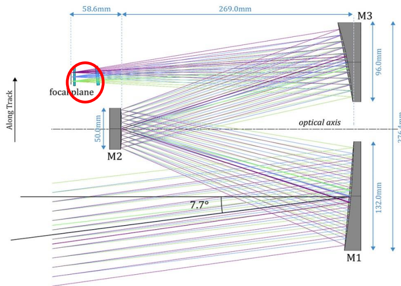
Fig.6 Layout of Janus; the spectral filter position is marked in red.
