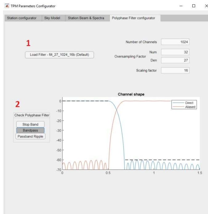
Figure 4: TPM secondary panels for the configuration of the polyphase filter
