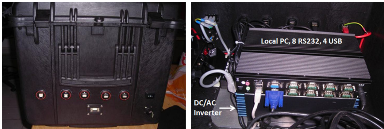
Figure 2. The Illuminator Control Box: on the left panel the exterior view showing the connectors for external interfaces; on the right panel the inside view showing the local PC used to interface and control the light generation and auxiliary devices.
