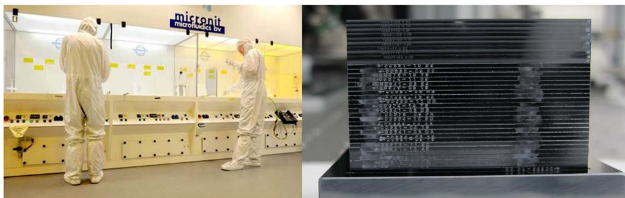
Figure 4: SPO mirror plates, already during the SPO development phase, being produced in industrial facilities (left). Each mirror plate is identified with a unique laser-engraved code, meeting the quality assurance requirements expected for the flight programme (right). Teledyne Imaging is being developed as a second, independent, mirror plate supplier, providing a robust supply chain for the future flight model implementation. Note in the right figure, that the mirror plates of the two suppliers are compatible with each other, being able to be stacked and bonded to each other (10 Teledyne Imaging plates bonded to 25 Micronit plates).
