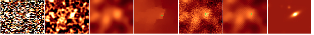
Fig. D.6. VIS crops visual comparison: Original, PSF, Perona-Malik, TVL2, bilateral, TV Chambolle, noiseless. The green boxes are the detected objects regions. The central object has been detected with a S/N of 21.26 with magnitude of 26.48.
