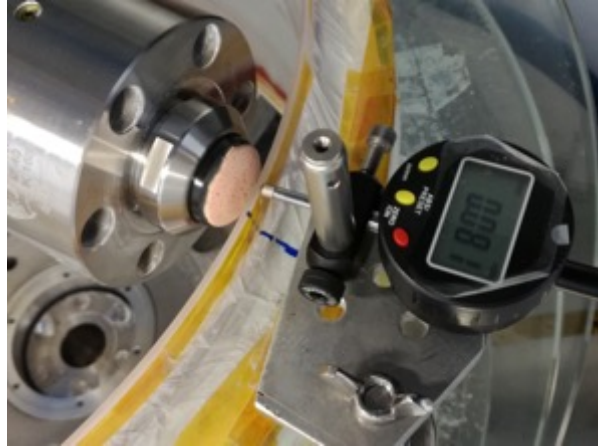
Figure 3: (A) The comparison between Bonnet tool R20 and R40. (B) The procedure to determine the offset to be applied.
