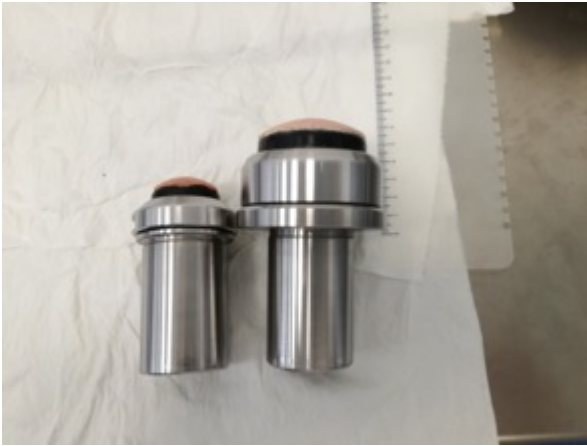
Figure 3: (A) The comparison between Bonnet tool R20 and R40. (B) The procedure to determine the offset to be applied.
