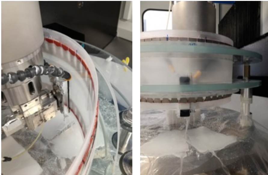
Figure 7: The pitch tool equipped with TRizact 3M™ is fixed on the robotic arm of the Zeeko machine and the vertical carriage movement has been used to move the tool up and down.
