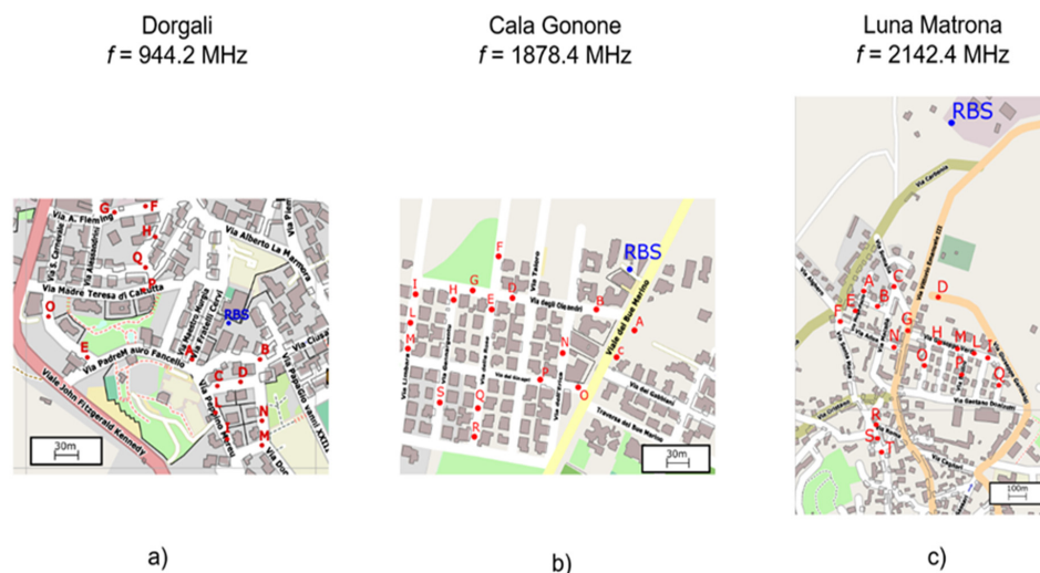
Figure 6. Topology of the three sites for the measurement campaigns. (a) Dorgali (NU, Italy): the working frequency of the RBS is 944.2 MHz, for a Kathrein 730376 antenna located 20 m above the road level. Fifteen measurement points were selected (A–Q). (b) Cala Gonone (NU, Italy): the working frequency of the RBS is 1878.4 MHz, for a Kathrein 742212 antenna located 10 m above the road level. Seventeen measurement points were selected (A–S). (c) Lunamatrona (CA, Italy): the working frequency of the RBS is 2142.4 MHz, for a Kathrein 742212 antenna located 30 m above the road level. Eighteen measurement points were selected (A–T).
