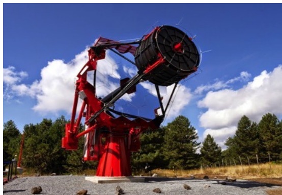
Figure 6: Left - The ASTRI telescope realized by INAF as prototype for the SST of the CTA observatory. Right - Diameter containing the 80% of photons as a function of field angle. Values are reported for the design (solid curve) and as measured at ASTRI telescope (dashed curve). The dimension of the SiPM pixel size (dashed horizontal line) and CTA requirement (solid horizontal line) are also shown for reference.
